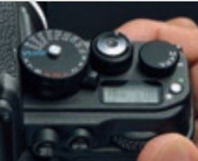
When set to 1/3 STEP, shutter speed can be controlled via the main command dial without taking your eye from the viewfinder
